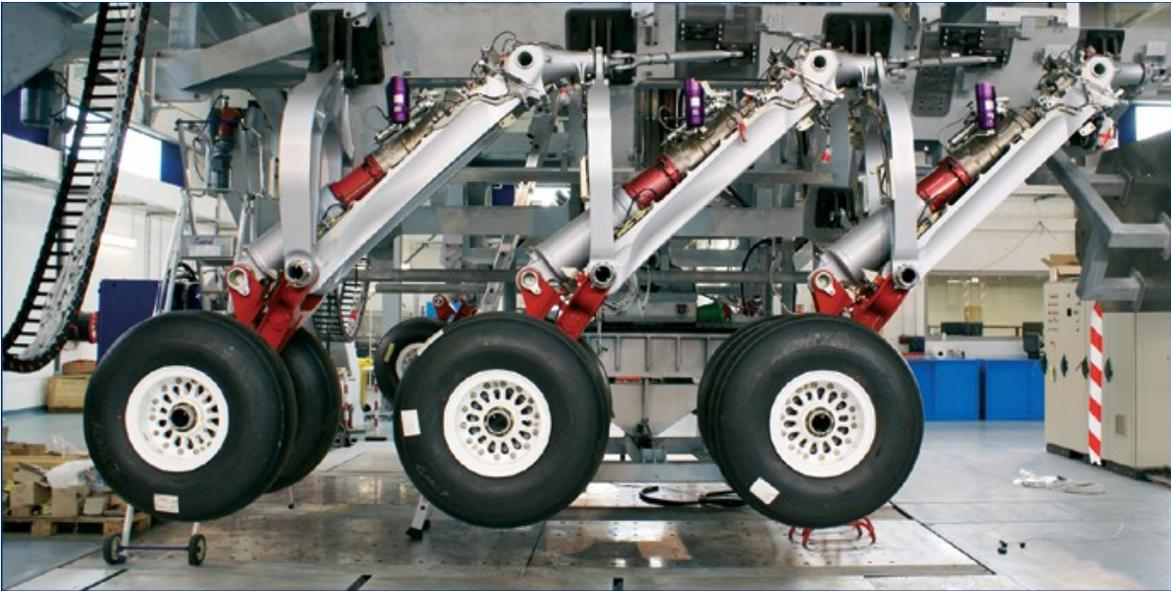
Starboard Main Landing Gear assembly at Vélizy
